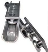
DEFENDER LINEAR RAIL® offers a rail and carriage block manufactured from 300 series stainless steel. Rollers are sealed, lubricated with mineral oil and manufactured from 440C stainless. The center roller is an eccentric allowing for preload adjustment.
